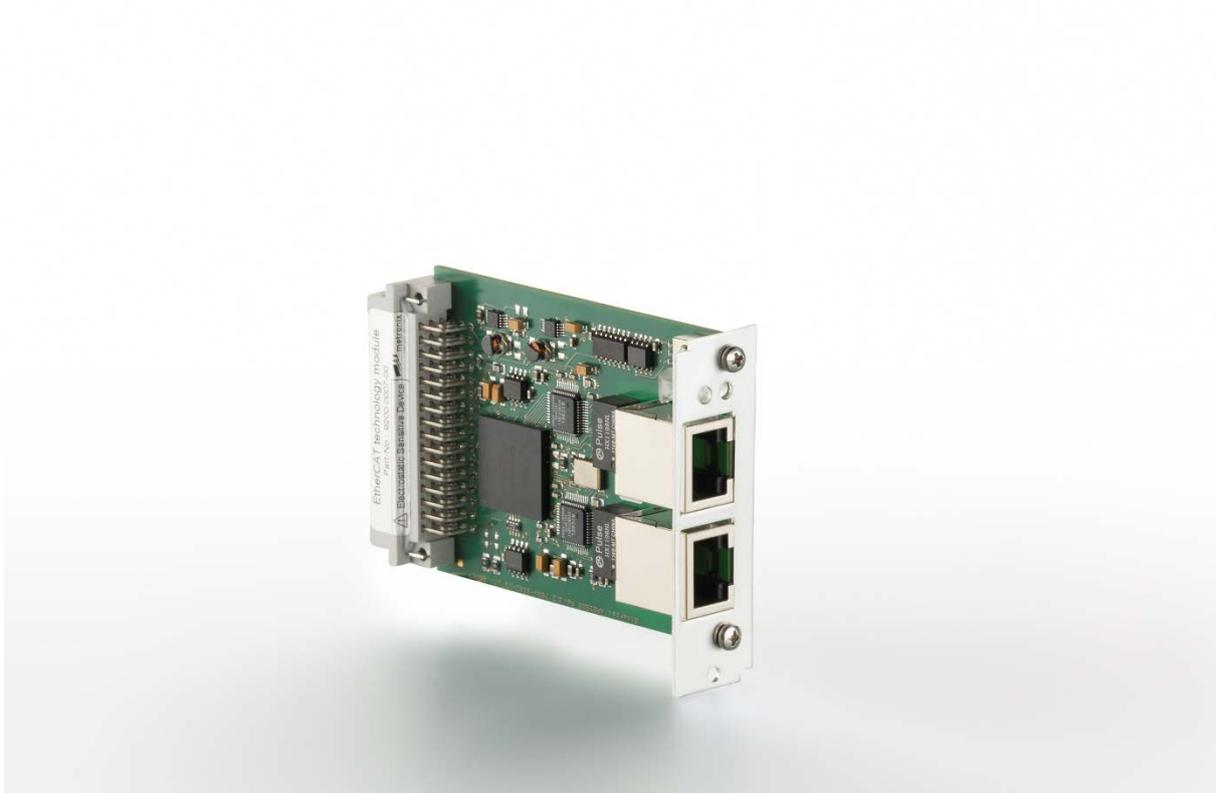
Figure 32: EtherCAT module: front view
